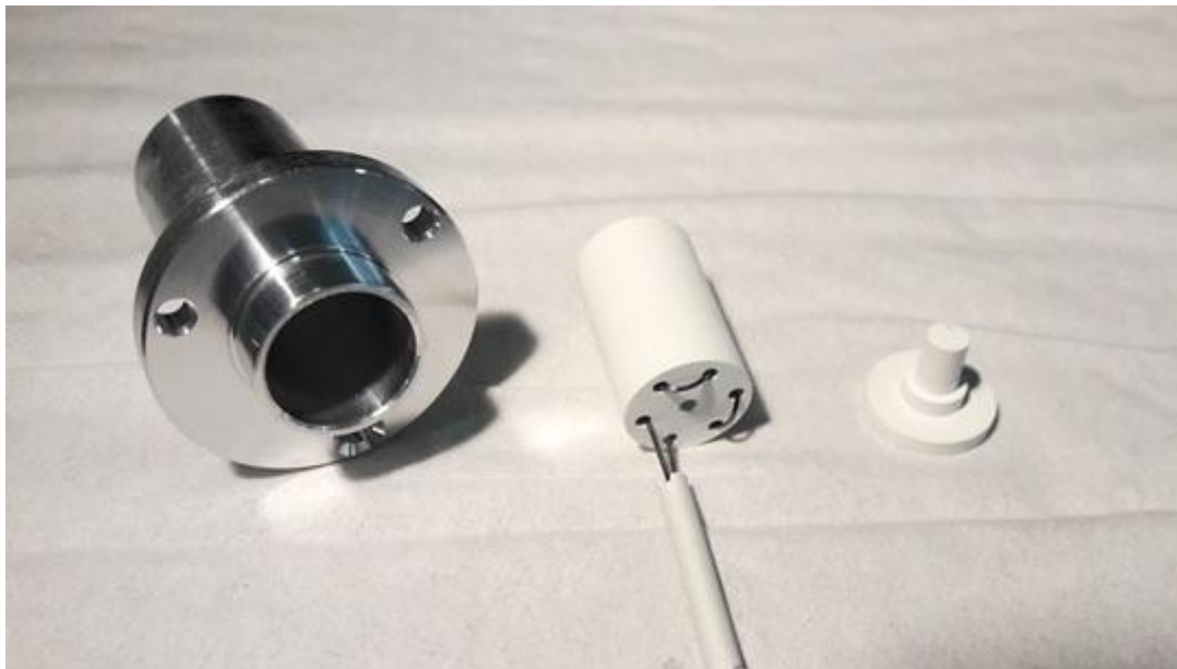
Figure 12: Top: In blue, Mass Marker or gas leak capillaries used for chemical traces injection in the target container or in the transfer line. Bottom: Heater assembly for reactants with low boiling point. From left to right: Aluminum case, heating cartridge: boron nitride insulating the tantalum heating wires and contains the sulfur powder, plug.
