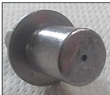
Figure 4. Optimized cathode after \approx 40 heating - cooling cycles and \approx 300 working hours at 2200 °C.
