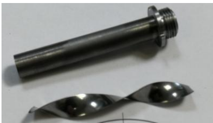
Figure 7: photograph of the transfer tube and associated helical chicane.
