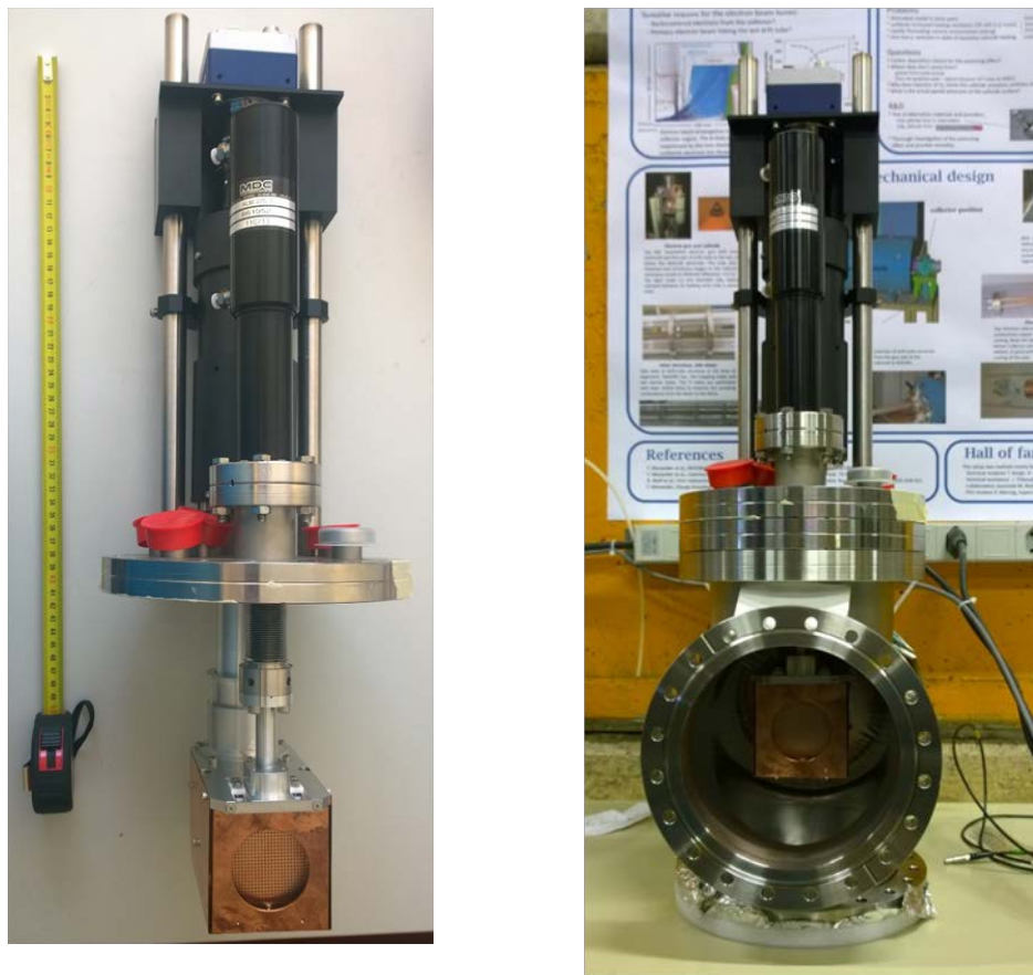
Figure 9. Assembled PPEM (left) and PPEM in the vacuum chamber prepared for tests (right).
